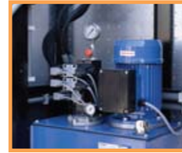
The hydraulic system is fitted with a number of safety locks and security precautions. An audio signal warns when opening and closing the doors.
